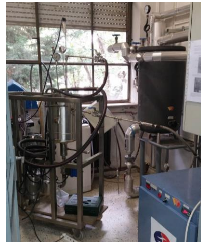
Fig. 1 Pilot scale plant of steam explosion.
