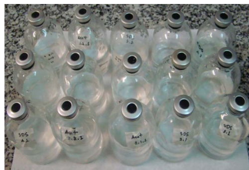
Figure 3. Batch cultures of SDS degrading microorganisms, under anoxic conditions.
